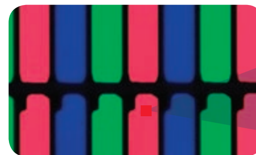
Image and transmission spectrum of LCD color mask pixels.
