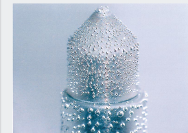
Electrode of xenon arc lamp (175x)
