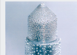
Electrode of xenon arc lamp (175x)
